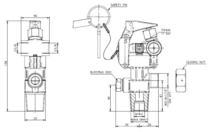
CLOSING NUT TO BE ALWAYS TIGHT TO THE VALVE OUTLET DURING TRANSPORTATION AND STORING UNTIL CO2 CYLINDER IS READY TO MOUNT INTO SYSTEM
