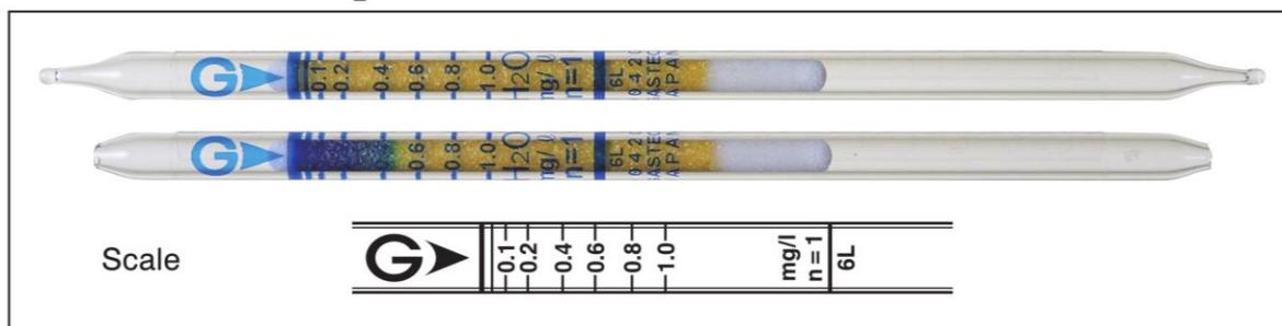
**Performance** The minimum scale value (0.05mg/L) is not printed on the tube, but only the scale line is printed.
