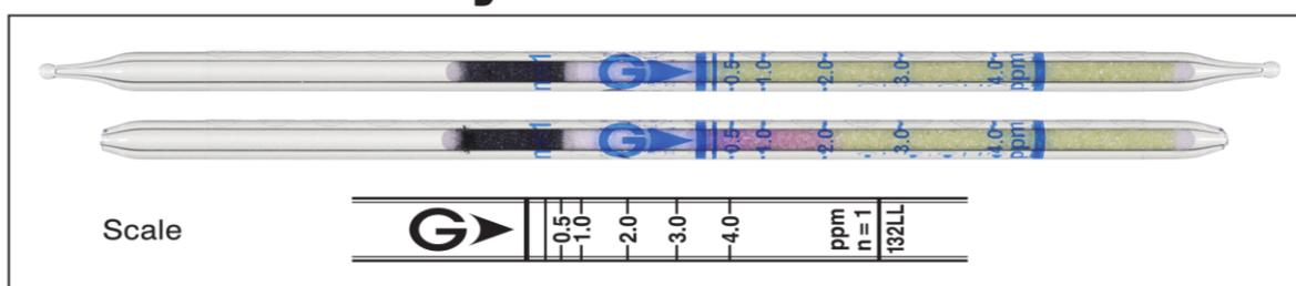
**Performance** The minimum scale value (0.25ppm) is not printed on the tube, but only the scale line is printed.
