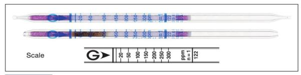
**Performance** The minimum scale value (10ppm) is not printed on the tube, but only the scale line is printed.
