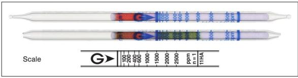
**Performance** The minimum scale value (50ppm) is not printed on the tube, but only the scale line is printed.
