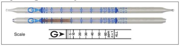
**Performance** The minimum scale value (2.5ppm) is not printed on the tube, but only the scale line is printed.
