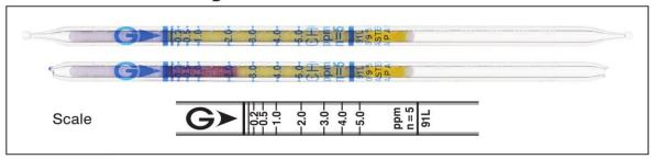
**Performance** The minimum scale value (0.1ppm) is not printed on the tube, but only the scale line is printed.
