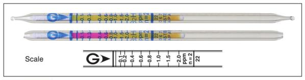
**Performance** The minimum scale value (0.05ppm) is not printed on the tube, but only the scale line is printed.
