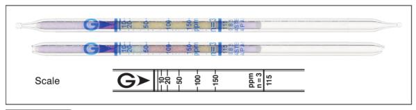
**Performance** The minimum scale value (5ppm) is not printed on the tube, but only the scale line is printed.
